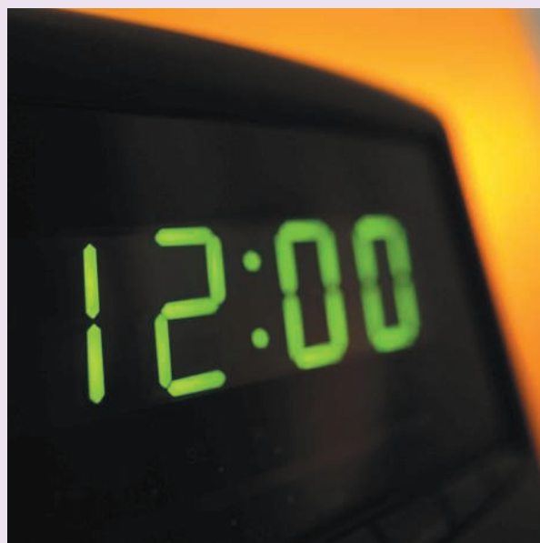
Each number in this digital display is made up of seven LEDs, each of which can be either 'on' or 'off'.
