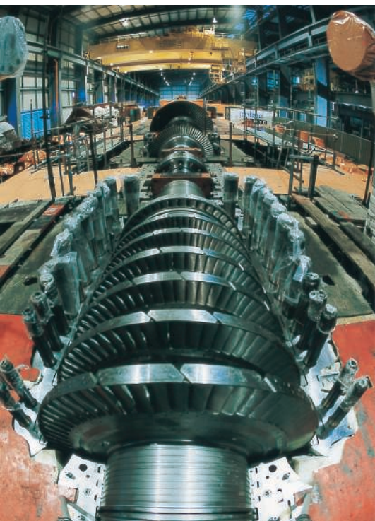
A 500 MW superheated steam turbine generator during construction
