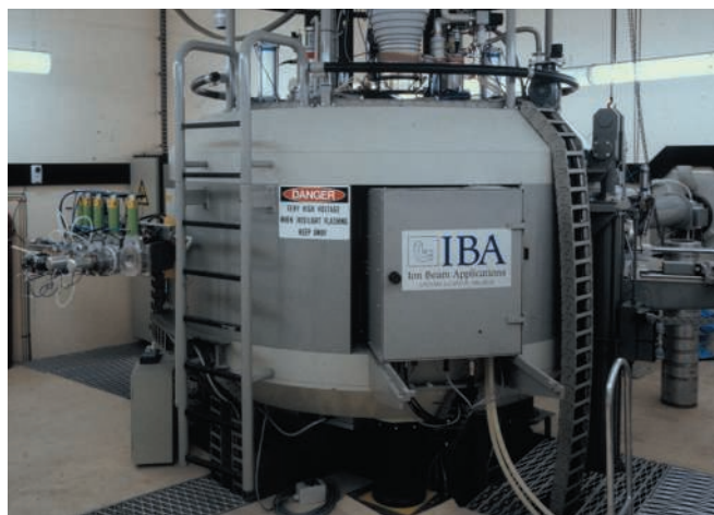
The National Medical Cyclotron in Sydney is used to make radioisotopes for use in hospitals.
